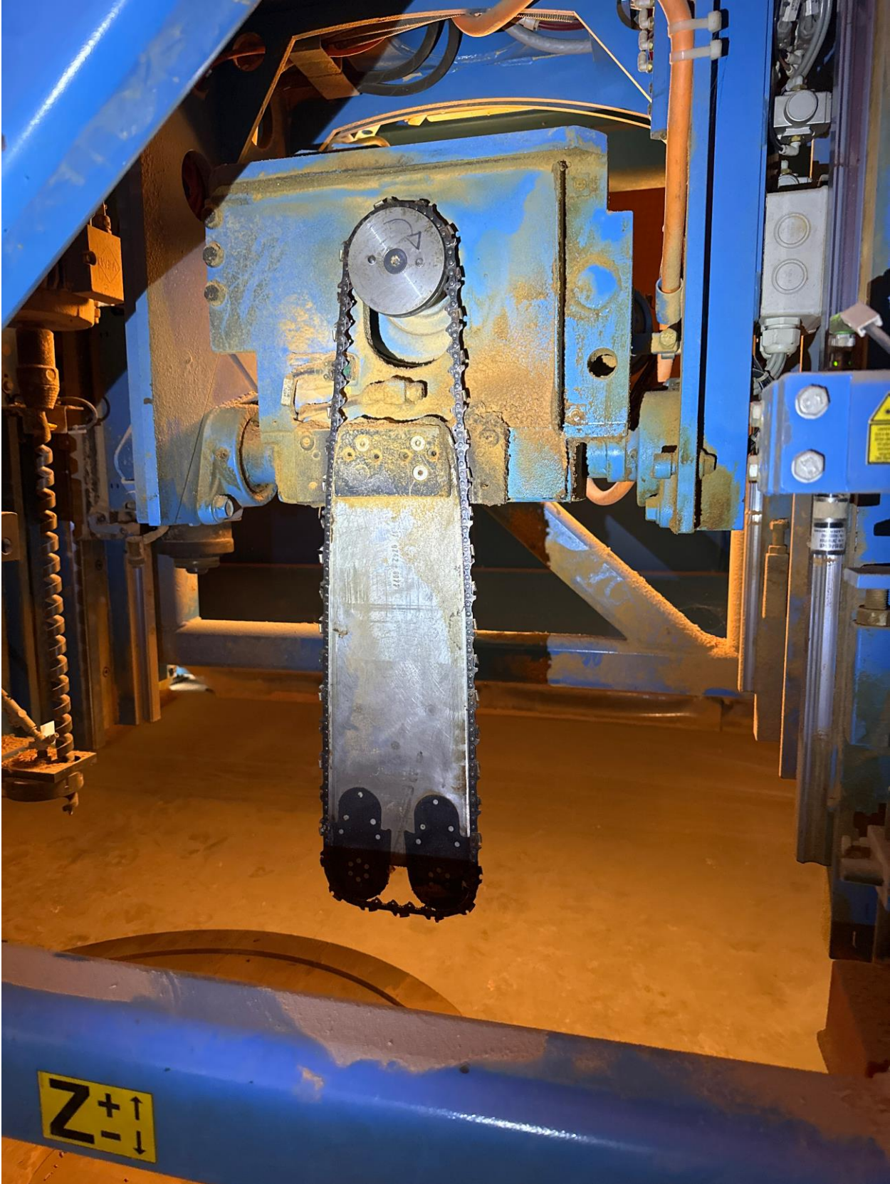
Chainsaw unit. Appears to be outfitted with the 20 inch bar and standard 3/8 inch chain.
