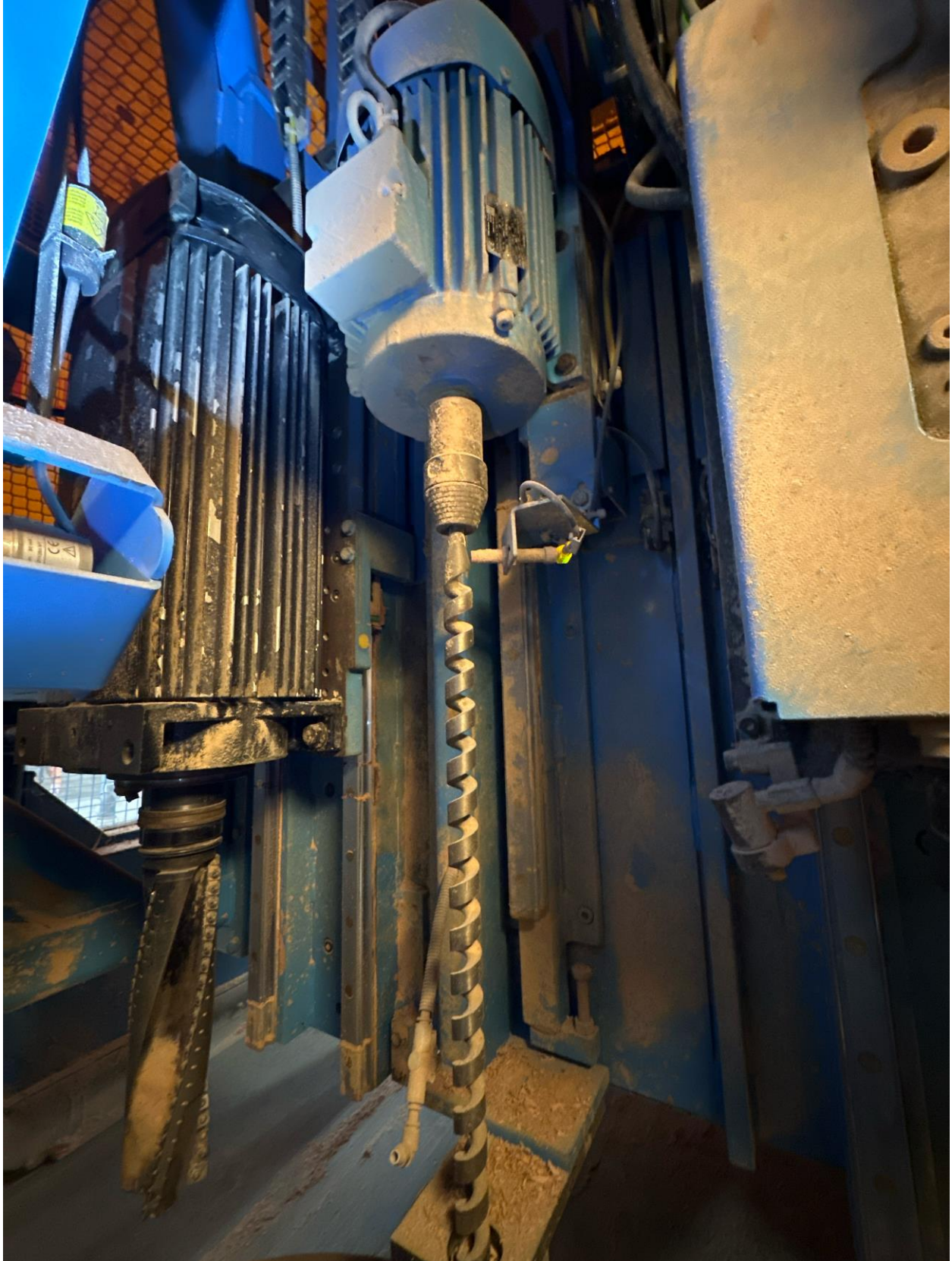
22 kW vertical milling motor with HSK 80 manual chuck
