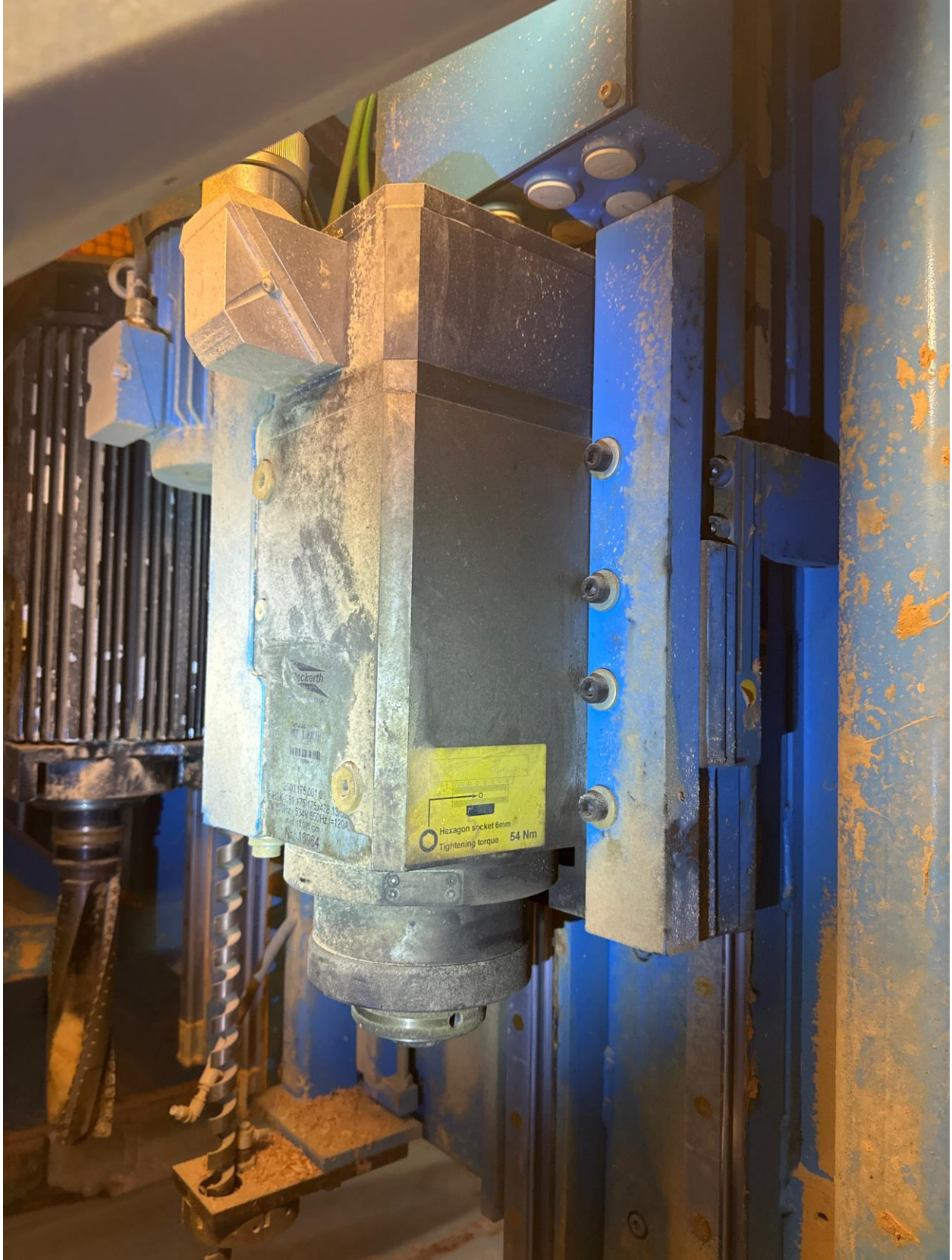
Pneumatic drill unit with a 3 kW drive motor
