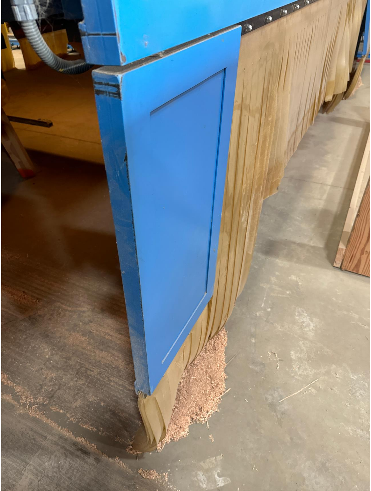
The left side rear panel is also fairly bent out of shape.
