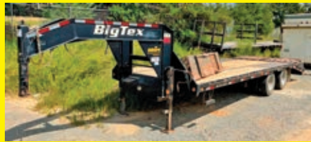
2018 BIG TEX 22GN-20BK+5MR SN:16VGX2028J6092162 equipped with 23,900 GVWR, 20ft. deck, 5ft. beavertail, steel ramps, 102in. wide, 48in. spread axle, ST235/80R16 tires, dual wheel, tandem axle.
