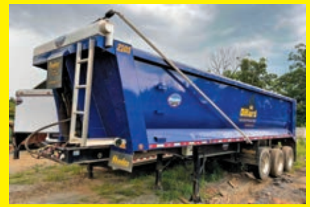
2019 RHODES WARRIOR RSS3260-3 VN:1A9SD3236KP432903 equipped with 32ft. length, 80,000 GVWR, roll tarp, dual rear gate, air ride suspension, 11R22.5 tires, air lift axle, triaxle.
