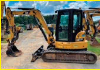
2019 CAT 305E2CR SN:H5M09850 powered by Cat diesel engine, equipped with Cab, air, front blade, swing boom, auxiliary hydraulics, rubber tracks, Cat coupler, digging bucket w/ hydraulic thumb, 1,019 hours.
