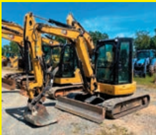
2020 CAT 305E2CR SN:H5M12524 powered by Cat diesel engine, equipped with Cab, air, front blade, swing boom, auxiliary hydraulics, rubber tracks, reduced tail swing, Cat coupler, digging bucket w/ hydraulic thumb.
