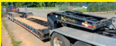
2016 KAUFMAN FR55DT-25K-43 SN:5VGFR433XGL003835 equipped with 134,000lb GVWR, non-ground bearing, 26ft. deck, 102in. wide, outriggers, air ride suspension, rear wheel covers, 275/70R22.5 tires, 2-air lift rear axles, fixed quad axle.
