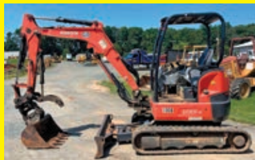
2019 KUBOTA U35-4 SN:12649 powered by Kubota diesel engine, equipped with OROPS, swing boom, auxiliary hydraulics, 4-way push blade, rubber tracks, swivel coupler, digging bucket w/ hydraulic thumb, 1,442 hours.
