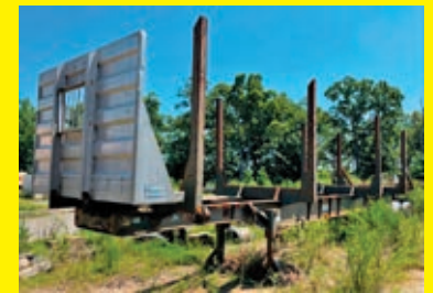
1998 PITTS LT42 VN:1PELT4228WP980370 equipped with 42ft. length, 95,000 GVWR, head rack, spring ride suspension, tandem axle.
