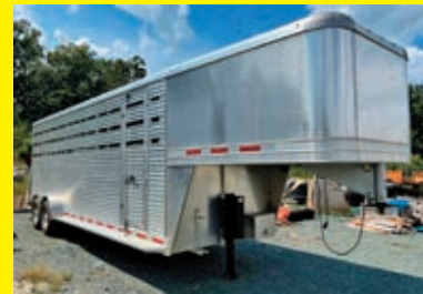
2019 ADAM JGA-247 VN:5CISG2420KR006372 equipped with 14,000lb GVWR, 24ft. body, 7ft. width, side door, dual rear door, ST235/85R16 tires, single wheel, tandem axle.
