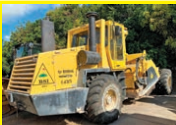
BOMAG MPH122 SN:90061074 4x4, powered by Deutz diesel engine, 482hp, equipped with EROPS, air, heat, 84.5in. Rotor width, 750/65R26 rubber, 3,087 hours.
