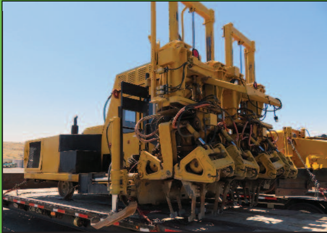
Jackson 2600 Tamper Ballast
