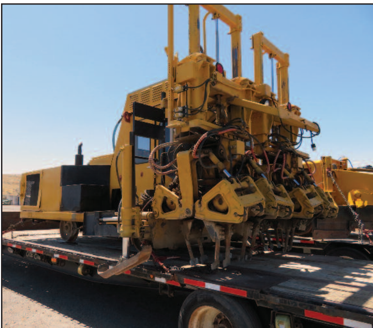
Jackson 2600 Tamper Ballast
