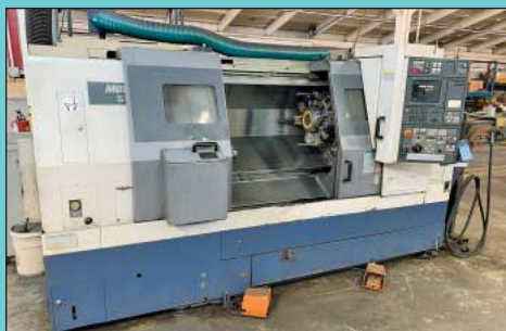
Mori Seiki Model SL-253 BSMC/1000 CNC Turning Center w/ Live Tooling & Sub Spindle
