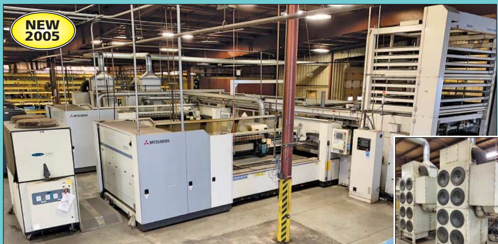
(2) 4,000-Watt Mitsubishi Model ML3015LVP (S) Plus CO2 Lasers w/ MSCiii-3015 Sheet Loader
