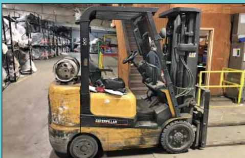
(2) 5,000 Lb. Caterpillar Model GC25K LP Gas Pneumatic Lift Trucks
