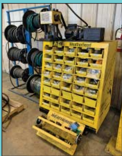
Coll-O-Crimp I Model T-400 Hose Crimper w/ Dies & Fittings
