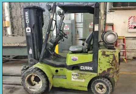
5,000 Lb. Clark Model CGP25 LP Gas Solid Pneumatic Tire Lift Truck
