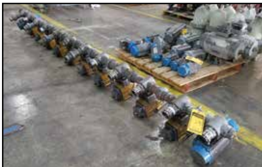
Pipe Valve Fixtures w/Actuator Valves
