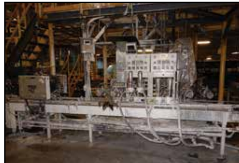
NEUPAK Twin-Lane 4-Head Quart Filler & Closer Line
